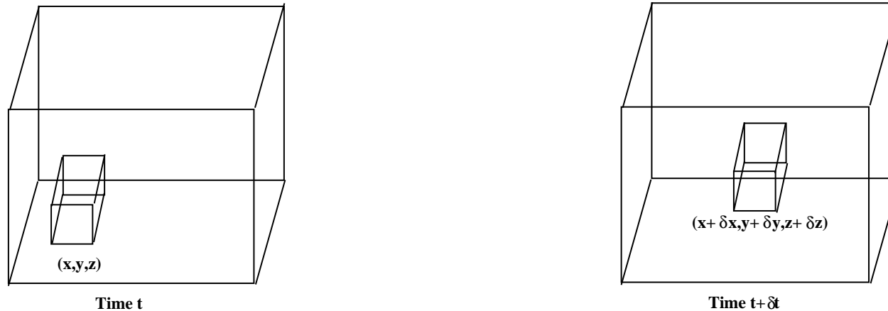
Figure 6: A small n \times n \times n 3D neighbourhood of voxels centered at (x, y, z) at time t moving to (x + \delta x, y + \delta y, z + \delta z) at time t + \delta t .
